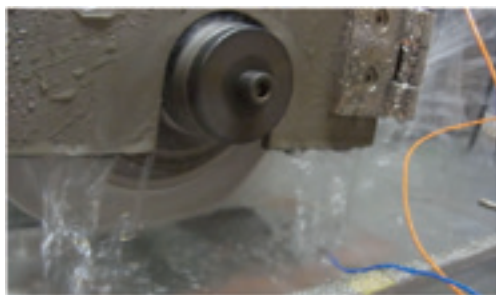
Situation of Water Machining *5) (Surface grinding, on-site prototype machine)
