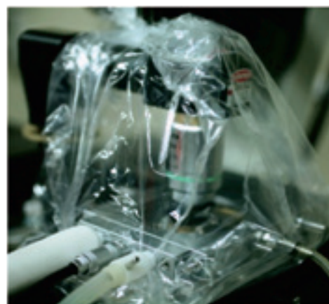
An imaging system which allows us to observe living cells under low-temperature and freezing conditions has been developed in Iwate University
